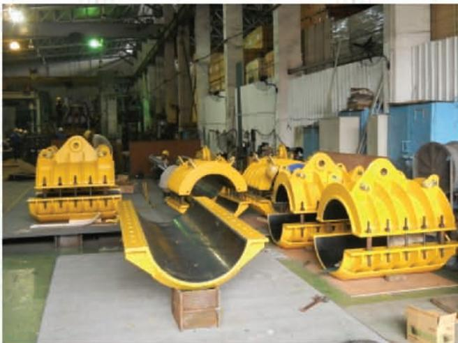
**Fabrication of Lifting Clamp and Anchor Clamp**
