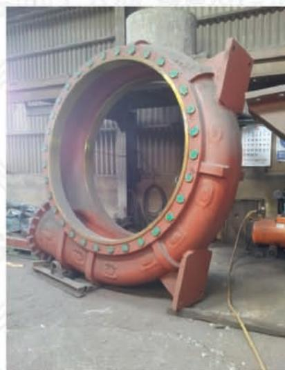
**Casting for Pump Casing**
