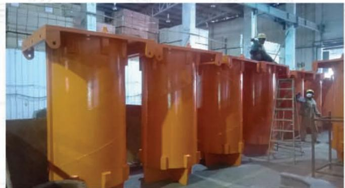
**Fabrication of Piling Sleeve and Support Beam Clamp**
