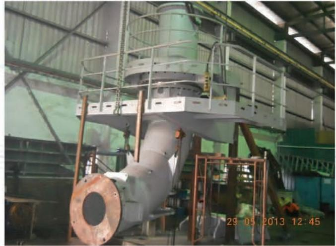
**Fabrication and Casting of Swivel Bend**
