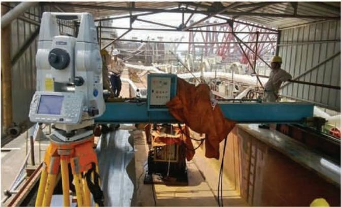
**Laser alignment using Total Station**
