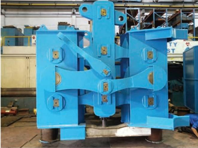
**Fabrication of Hoisting & Holding Clamps**
