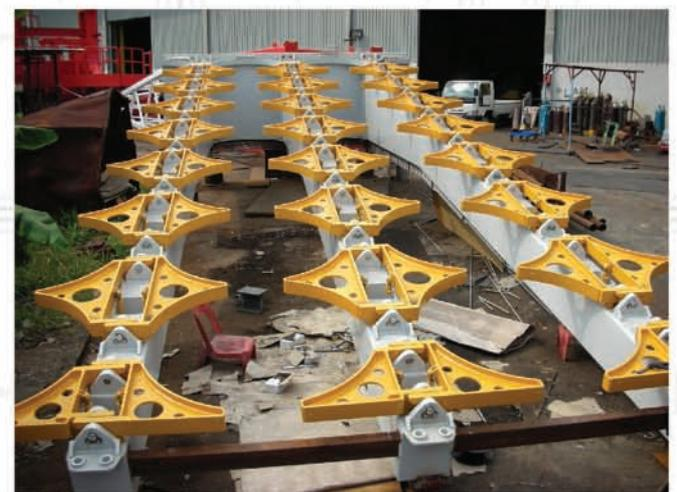
**Complete Fabrication of Offshore Drilling Equipment (Riser Fingerboard) with Installation and Hook-Up Service**
