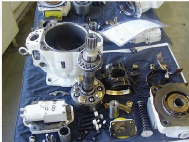
**Overhaul of hydraulic component (e.g. Motor, pump, and cylinder)**
